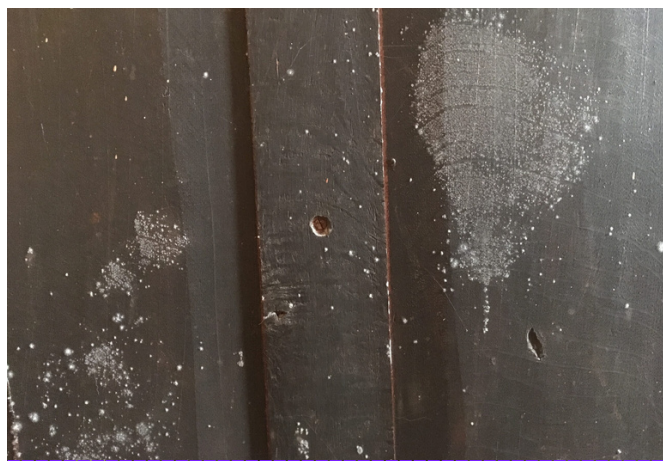
Fig. 1 — Mold growth on the back of wooden furniture. Photo: Morena Ferreira.
